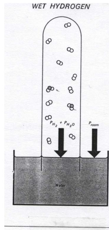
This was done to equalize the atmospheric pressure (room pressure) with the gas pressure ( $P_{\text{total}}$ ) inside the burette. At this point:
