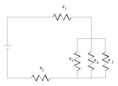
$R_1 = 25 \Omega$   $R_2 = 15 \Omega$   $R_3 = 20 \Omega$  $R_4 = 30 \Omega$   $R_5 = 60 \Omega$
