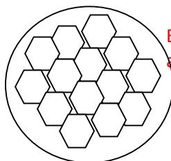
**Each honeycomb structure increases surface area and allows more Pt and Rh catalyst to be packed in.**
