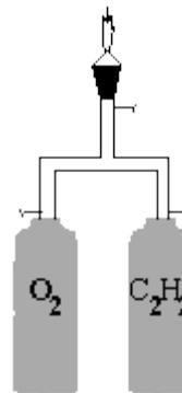
In an *oxyacetylene blow torch*, steel cylinders containing acetylene and oxygen are connected through hoses that join together, and then connect to a nozzle. The mixture is combusted and produces a flame capable of cutting through metal.
